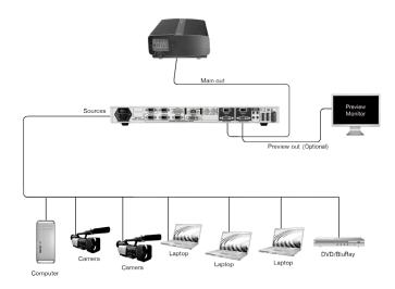
Connect all of your sources (PC, video camera, streaming server, DVD player...) to the appropriate input connectors at the rear of the unit (see "The SmartVu rear panel" p.22 of the User Manual).
